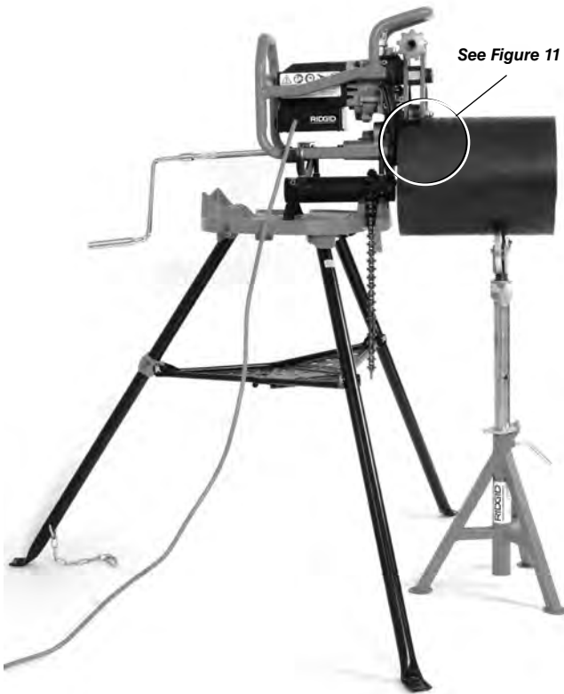
Figure 12 – Fixed Beveller, Short Pipe, One Pipe Stand
